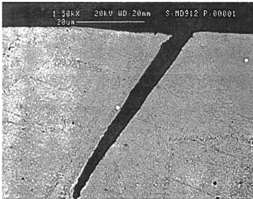
Figure 2 – SEM Backscatter Electron Image Showing Crack Formation Along a Slip Band (1.5 kX).
