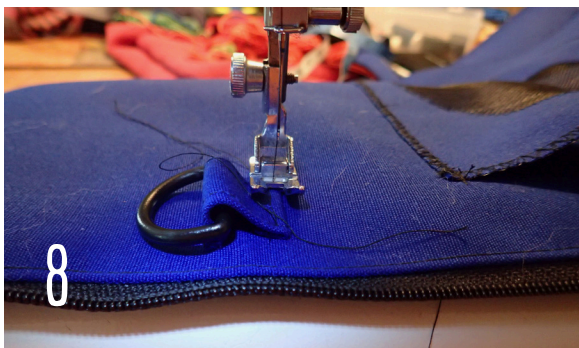
8 Use nylon webbing or make fabric tab to hold D-ring in place, centered over fold, just below zipper edge.
