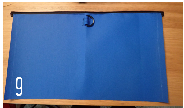
9 Use nylon webbing or make fabric tab to hold D-ring in place, centered over fold, just below zipper edge.
