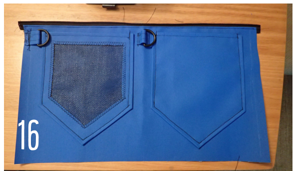
Stitch 2nd D-ring tab in place on seam allowance, matching position with center D-ring.
