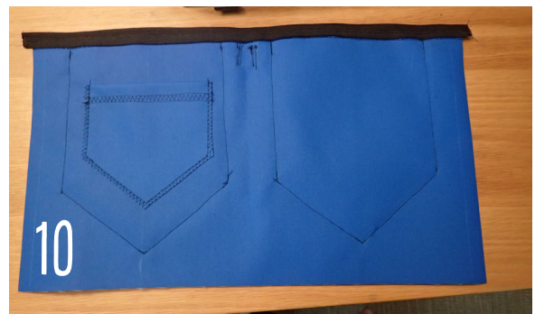
10 Zig zag edges of cut-out, fold over 1" and stitch down. Stitch interior pocket in place on back interior side.
