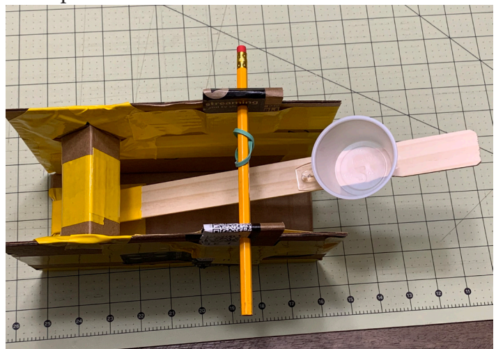
24) After checking placement of pencil and tab supports, tape tab supports in place.
