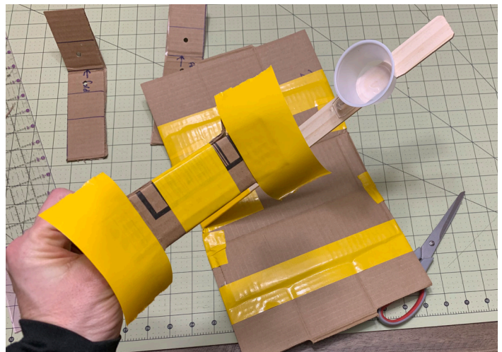
17) Cut two pieces of duct tape to attach to two tabs of cross-support as shown.
