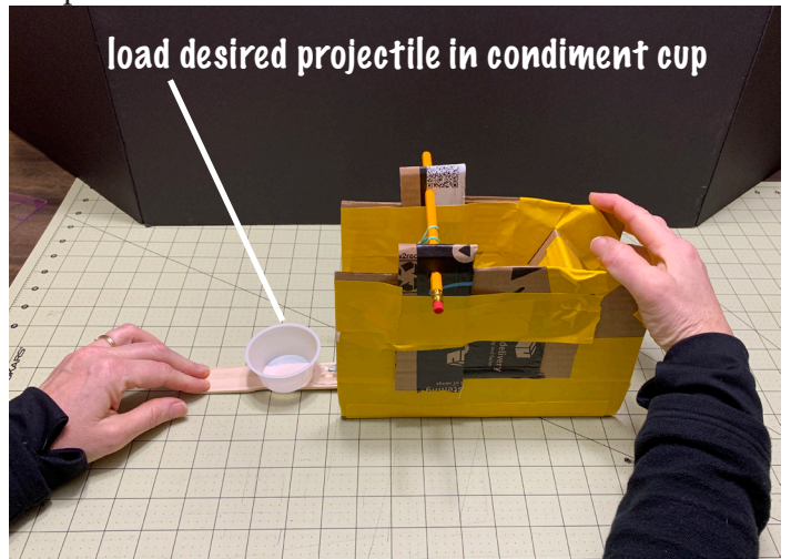
29) When the lever arm is flush with the ground, you're ready to launch (just release lever arm).
